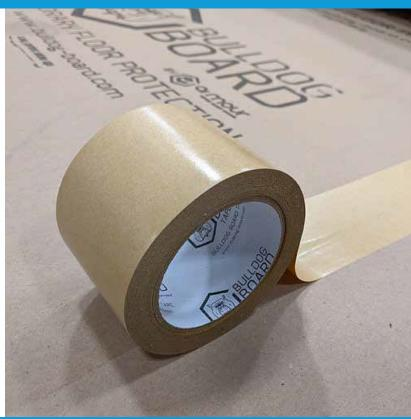
Bulldog Board Tape is a very tension resistant paper tape with high-tack adhesive, making it an excellent choice for seaming Bulldog Board and other paper based floor protection products together. This tape is designed to seam Bulldog Board together and should not be applied to a finished surface. For a clean removal solution, use Armour Tape.
