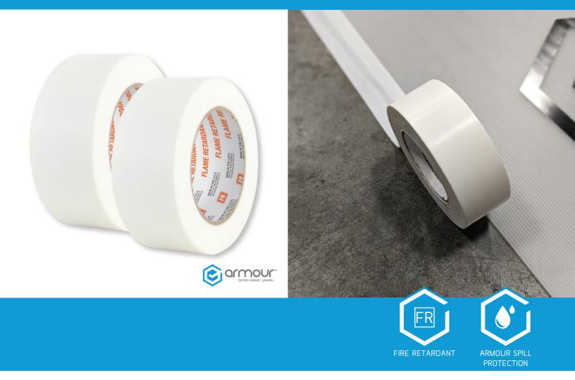
Armour Tape – FR is polyethylene backed and meets the fire test requirements of NFPA 701 standard and ASTM E84 for fire retardancy. This is an excellent solution for use with temporary surface protection products where there is high heat, sparks, or any other type of fire hazard. It bonds well to different surfaces over a wide temperature range, and allows for clean and easy removal.
